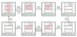
Example 1: The factory default parameter is AC 5A(CT=1); If the current transformer is 1000A/5A, should modify the CT multiplying power as 200(1000/5)
