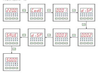
3.6.2 set multiplying power of current transformer is 100(CT 500A/5A)
