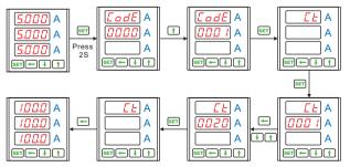
Example 2: The factory default parameter is AC 10KV/100V(PT=10KV/100V=100); If the voltage transformer is 10KV/100V, should modify the PT multiplying power as 350(PT=35KV/100V=350)
